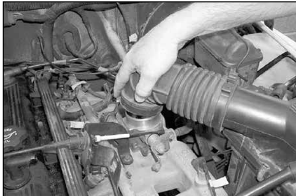
4. Loosen the hose clamp at the throttle body, then detach the stock intake tube from the throttle body as shown.
