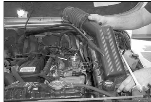
5. Unclip the three lower air cleaner retaining clamps, then remove the upper air cleaner assembly as shown.
