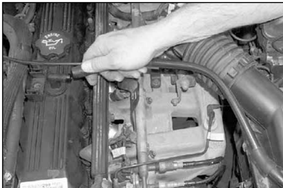
2. Disconnect the crank case vent hose.
